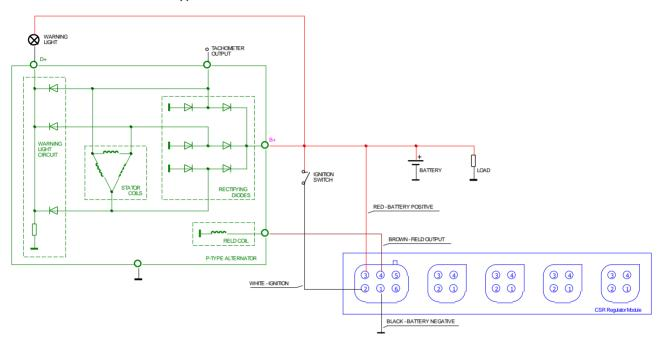
Reference schematic for N-type alternator
